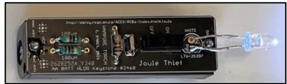
Switch: GND → Emitter and LED (PCB)
