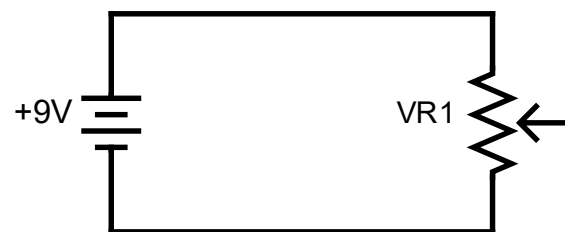
Figure 2. Variable voltage divider
