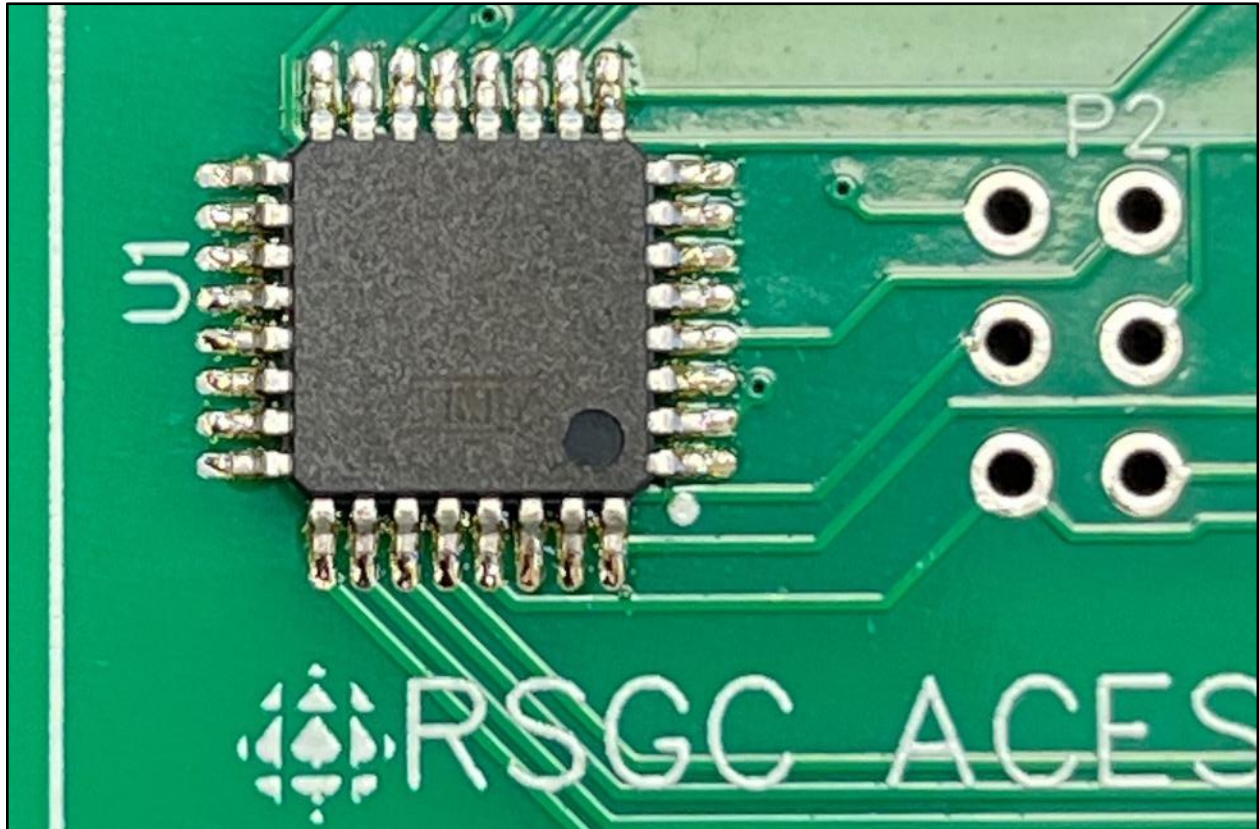
Solder Joints on Atmega328P on The Motherboard
