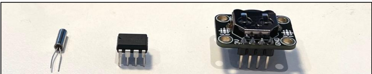
RTC (Middle) and Supporting Components Crystal (Left) and Battery Breakout Board (Right)
